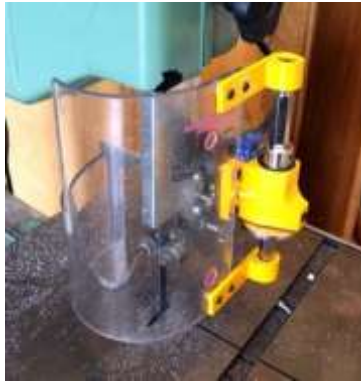
Vertical bandsaw guard with a non-contact safety switch
