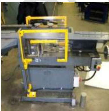
Horizontal bandsaw (sm) guard with (2) non-contact safety switches
