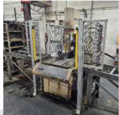
Vertical bandsaw (lg) guard with safety light curtains
