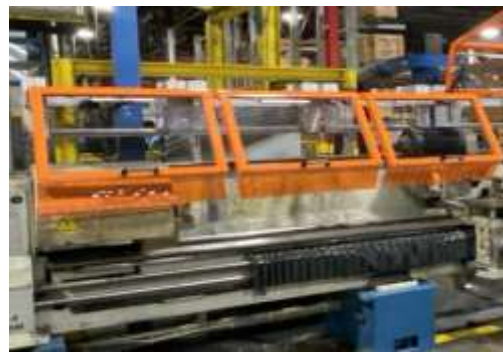
Large Lathe Guard with (x) non-contact safety switches
