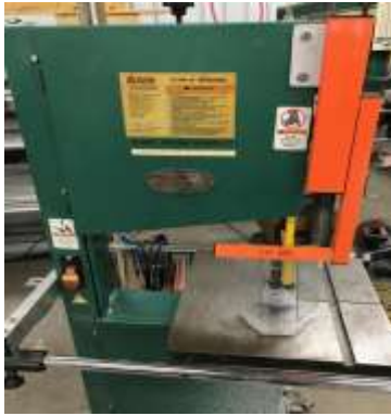
Vertical bandsaw (sm) guard without a safety switch
