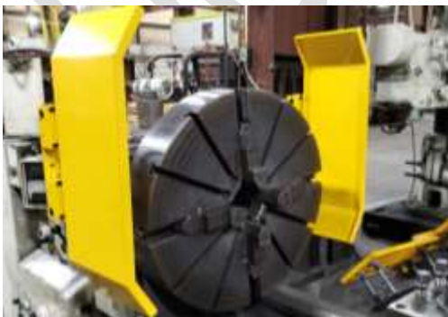
Large Lathe Guard with (2) non-contact safety switches
