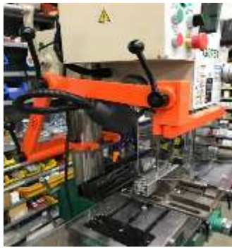
Drill press guard with a non-contact safety switch
