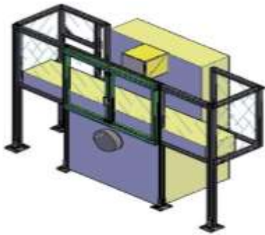
Floor Mounted Surface Grinder Guard without a safety switch
