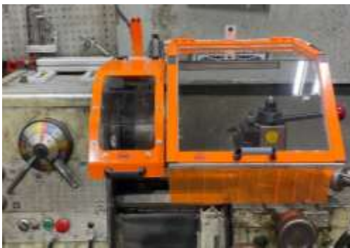
Chuck guard (primary) and lathe guard (secondary) with (2) non-contact safety switches and bypass key
