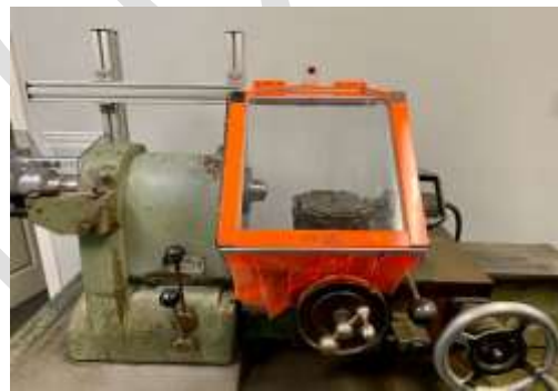
Hardinge lathe guard and collet closer with a non-contact safety switch
