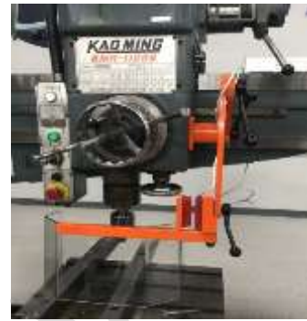
Radial arm drill with a non-contact safety switch
