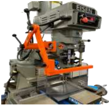
Head mount mill guard with a non-contact safety switch
